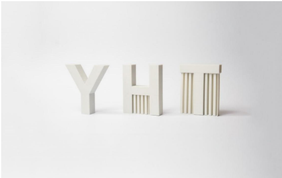
Figure 12. Lettres Y, H et T imprimées avec support (Source: https://www.hubs.com/knowledge-base/supports-3d-printing-technology-overview/ )
