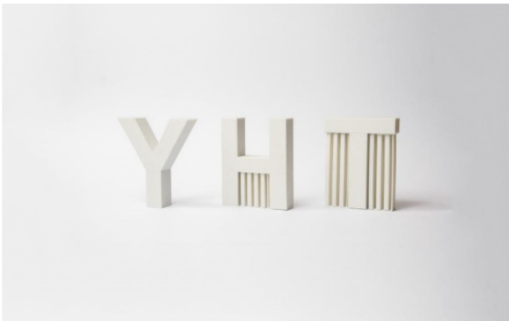
Figure 12. Letter T printed with and without support material (Source: https://www.hubs.com/knowledge-base/supports-3d-printing-technology-overview/ )
