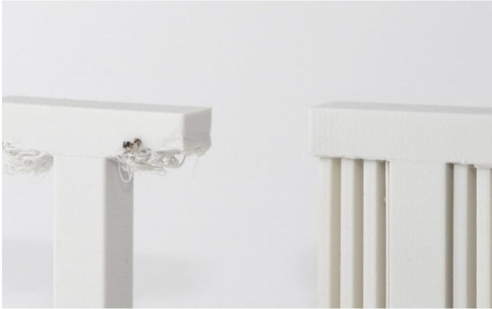
Figure 11. Letters Y, H, and T printed with support material (Source: https://www.hubs.com/knowledge-base/supports-3d-printing-technology-overview/ )
